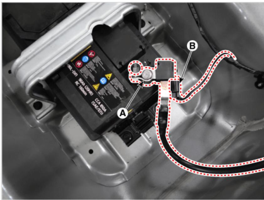
6. Remove the battery sensor by loosening the mounting bolts (A).
